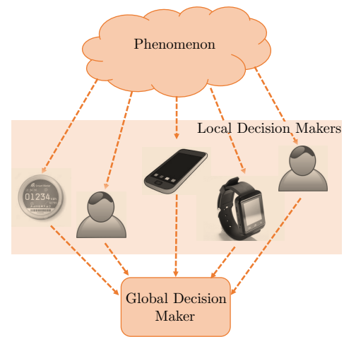
Fig. 1. System model consisting of local decision makers and a global decision maker.
